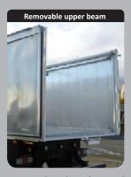
Upper beam that can be removed provide integral clearance.
