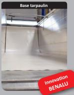
Base tarpaulin equipment designed to ease the flow of products that are sticky and ensure total safety (Patent no. FR2976532)
