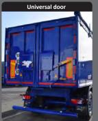
Universal door of various thicknesses closed by bolts and gate.
