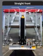
A straight front with external jack cylinder providing a volun extending to 89 m<sup>3</sup>
