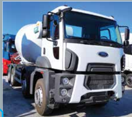
15.09.2021. - Slovenija FORD TRUCKS 4142 M with 9m³ concrete mixer upgrade
